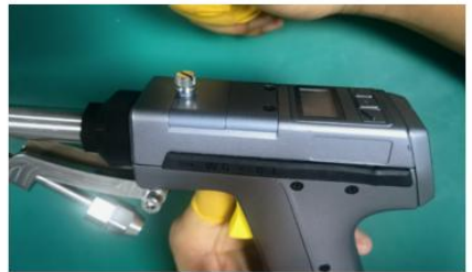
④ Replace the protective lens and install it
